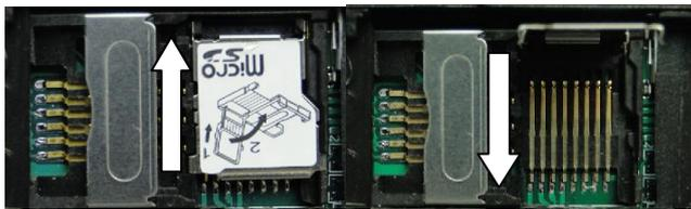
5.1.3 Put the SIM card into the holder as picture shows.
